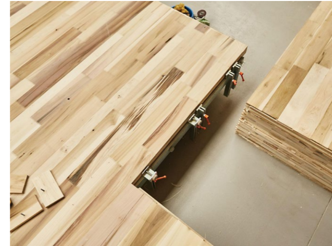
CLT panels in storage after removal from press
