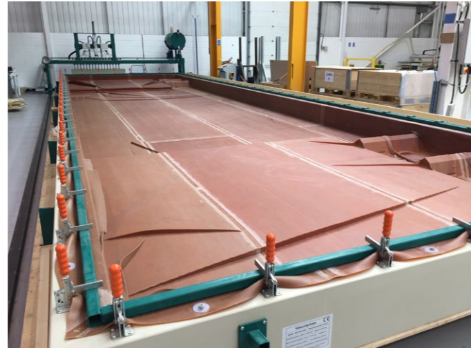
CLT panels under load in the vacuum press
