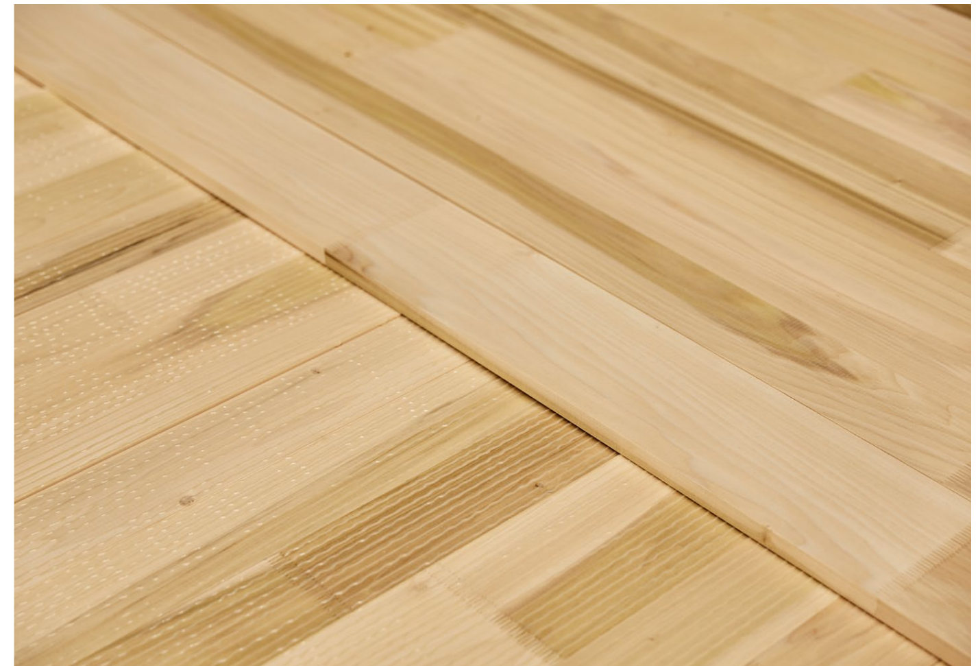
Close-up of tulipwood CLT panels
