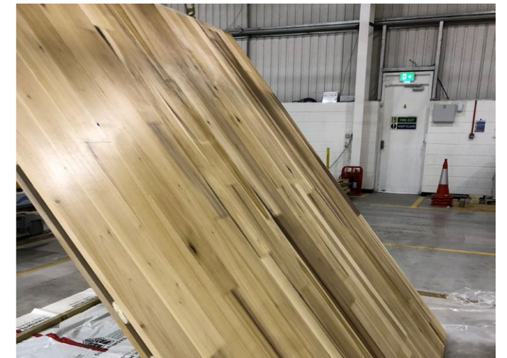
CLT panel sanded and lacquered
