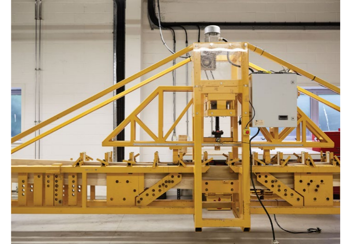
Edgewise bending testing at Edinburgh Napier University
