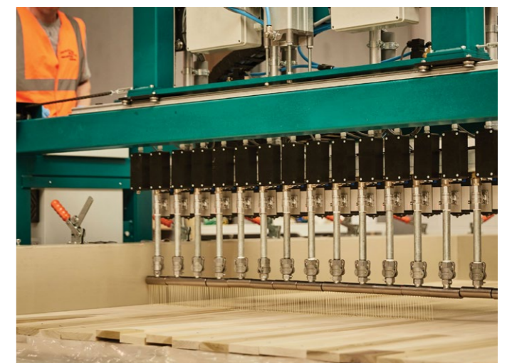
Application of adhesive during panel manufacture at CSIC
